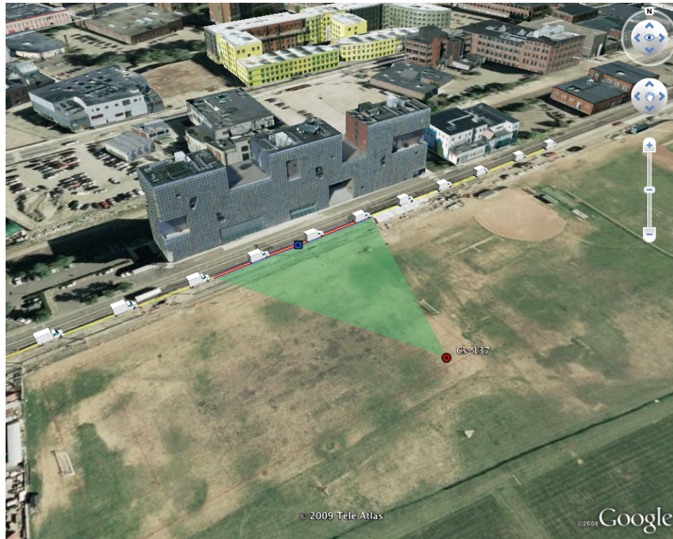
Figure 8.9: Google earth view of the located and identified source. The square symbol represents the average location of the TMI for the data used to image the source. The circle denoting the isotope ( ^{137}\text{Cs} ) is the reported geo-location and the path of travel is shown with the truck model. The shaded area shows the region of data used to image the source.
